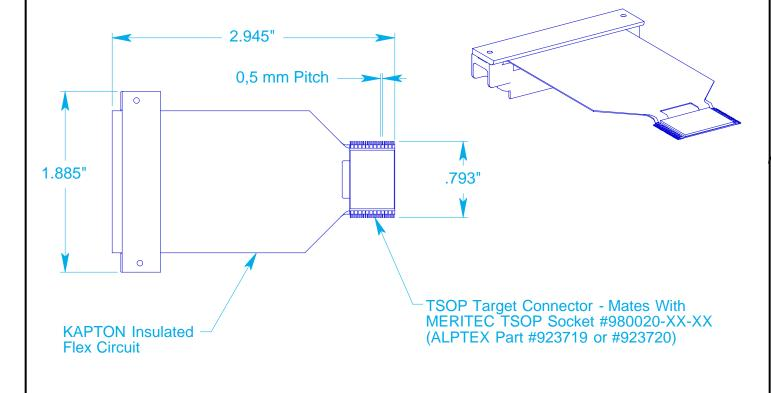
50 Position Interface Connector -Mates With MERITEC Surface Mount Hermaphroditic Connector (ALPTEX Part #923718-50)
