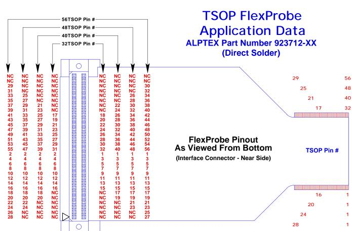
Note: This FlexProbe is designed to be reflow soldered directly to the P. C. Board.
