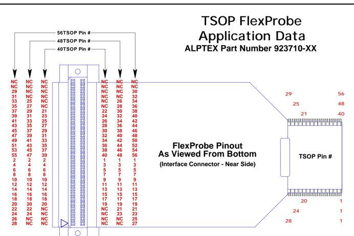
Note: This FlexProbe is designed to mate with MERITEC TSOP Socket #980020-XX-XX ONLY. It is not intended for use with other sockets or in solder down applications.
